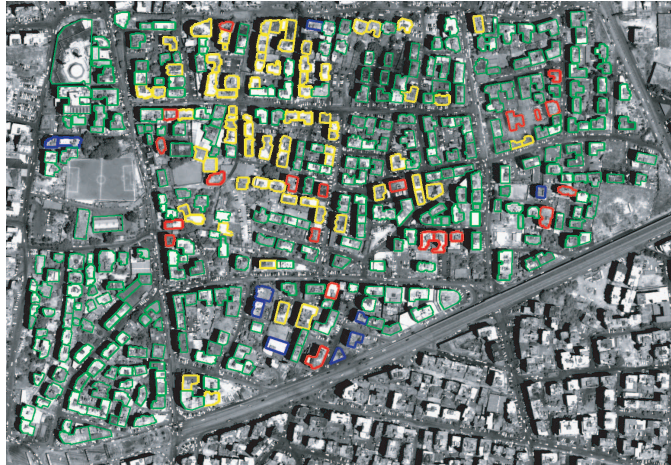
Figure 2: Area of Haret Hreik, in Beirut, Lebanon. Image acquired in 19 June 2006 (reference image). The footprints of the 430 buildings contained in the GIS, used as additional input, is overlaid. The green corresponds to intact or not detectable damage (325 buildings); the yellow to buildings destroyed between the 19 June 2006 and the 22 July 2006 (74 buildings); the red to buildings destroyed between the 22 July 2006 and the 9 August 2006 (21 buildings); the blue is for buildings destroyed between the 9 August and the 12 August 2006 (10 buildings).
